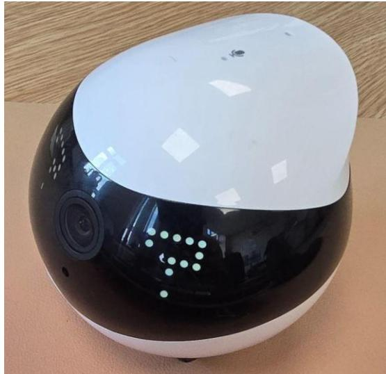
When the robot displays the question mark symbol then the student can't hear the lesson.
